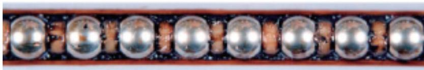
Ball cage after running 8,000 km (Test stop)
