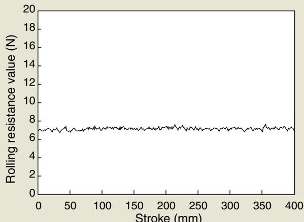
Results of Measuring Fluctuations in Rolling Resistance of SHS25LV (with ball cage)
