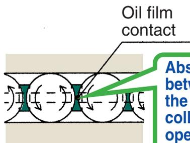
Absence of friction between balls eliminates the generation of collision noise for quiet operation
