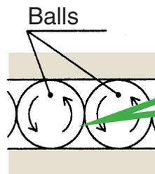
Friction occurs between balls resulting in the generation of collision noise
