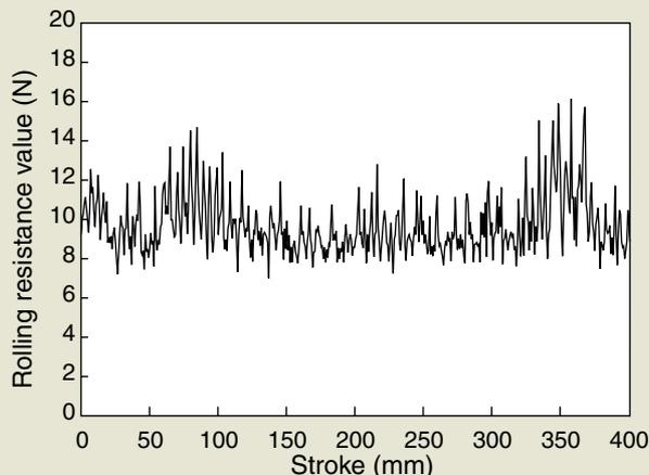
Results of Measuring Fluctuations in Rolling Resistance of HSR25LR (without ball cage)
