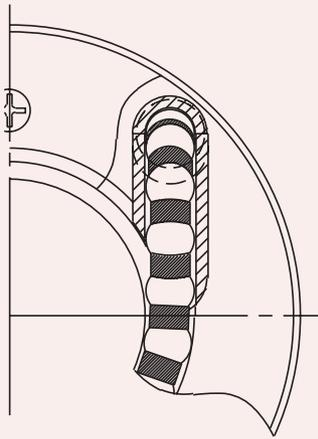
Balls circulate in the lead angle direction
