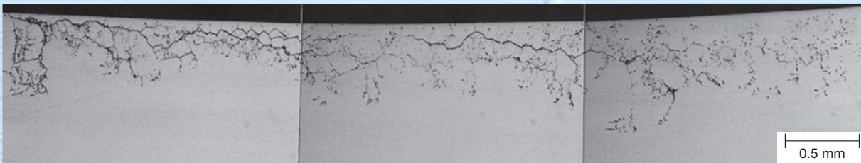
Photo 4. Cracks along grain boundary
