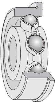
This type of miniature and extra-small ball bearings has a flange on one end of the outside surface.
