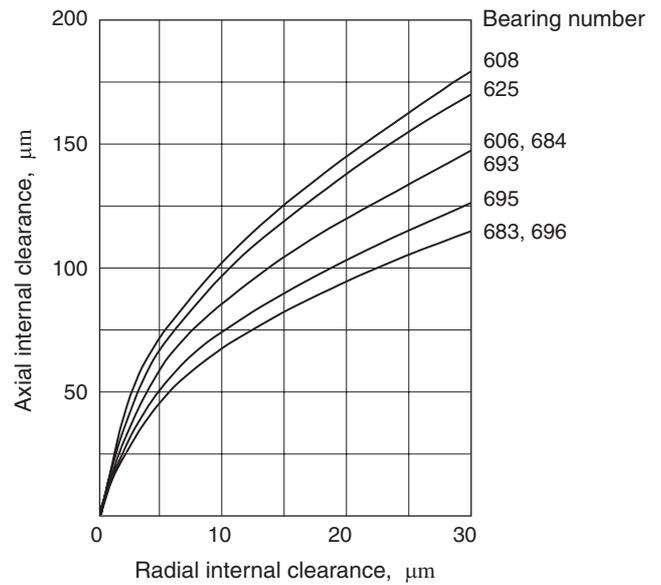
Fig. 6.2 Relationship between Radial and Axial Internal Clearance
