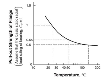
[Note] These values for the pull-out strength of flange are valid when an axial load is applied evenly to the whole circumference of the flange. If the load is applied locally, the C<sub>0r</sub> value may decrease by approximately 10% (C<sub>0r</sub> denotes the basic static radial load rating of bearing).
