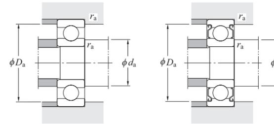
Dynamic equivalent radial load  $P_r = XF_r + YF_a$
