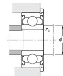
Dynamic equivalent radial load  $P_r = XF_r + YF_a$
