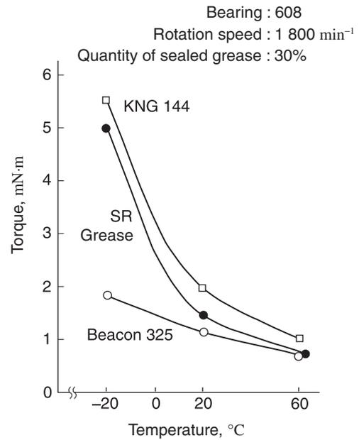
Fig. 9.2 Relationship between Temperature and Running Torque
