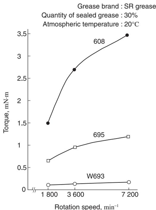
Fig. 9.1 Relationship between Rotation Speed and Running Torque
