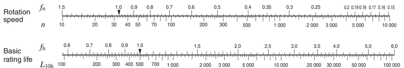
Fig. 2.1 Rotation Speed ( $n$ ) and its Coefficients ( $f_n$ ), and service Life Coefficient ( $f_h$ ) and basic rating Life ( $L_{10h}$ )
