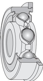
In this type of bearing a resin flange is injection molded around the outside surface, as an alternative to the solid outer ring flange.
