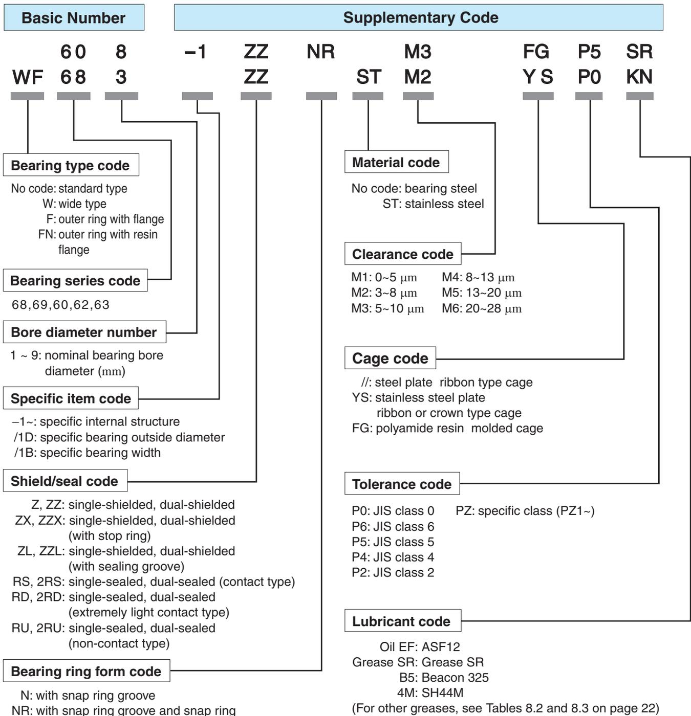
Table 1.3 Metric Series Miniature and Extra-Small Ball Bearings (Specific Dimension Series)
