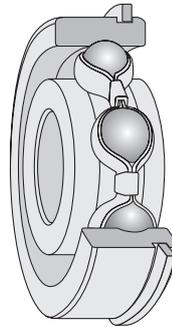
With this type of bearing, mounting in a housing is simple, as its positioning in the axial direction is carried out using a locating snap ring.
