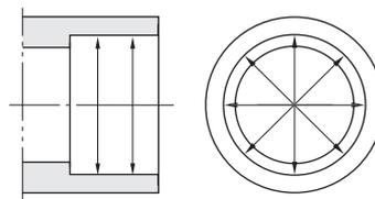
Fig. 11.2 Measuring Positions of Housing Bore Diameter
