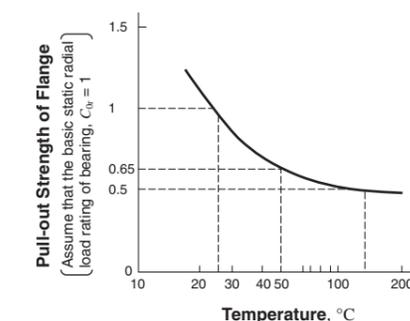
[Note] These values for the pull-out strength of flange are valid when an axial load is applied evenly to the whole circumference of the flange. If the load is applied locally, the C<sub>0r</sub> value may decrease by approximately 10% (C<sub>0r</sub> denotes the basic static radial load rating of bearing).
